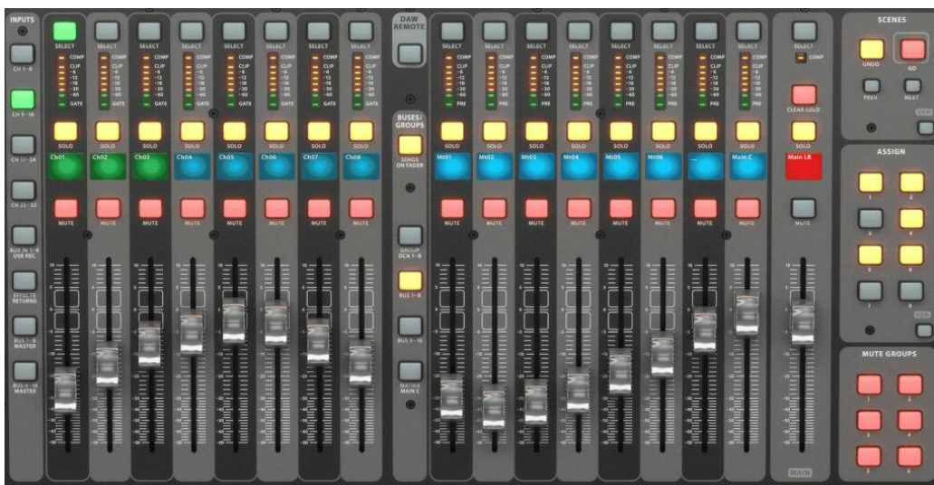
Poor gain structure causes faders to be inconsistent and far from unity
